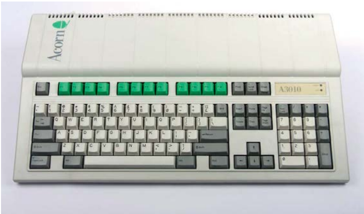
LEFT The English-made Acorn Archimedes A3010 was the first machine to use the now standard ARM computer architecture.
