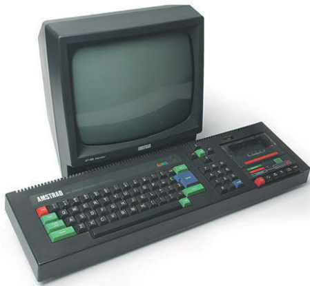
ABOVE The optional greenscreen monitor and tape-loader for the Amstrad CPC 464 was a big feature in a lot of childhoods.
